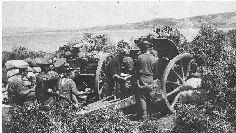
The Quick Firing (QF) 18 Pounder was the principal Field Gun of the British Army. It was towed by a team of six light draught horses and the calibre and shell weight made it most destructive.
