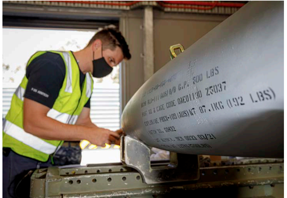
Armament Technician, Corporal Andrew Johnston from No. 3 Squadron, assembles a Guided Bomb Unit (GBU-12) using a new Australian manufactured Bomb Live Unit (BLU 111) at RAAF Base Williamtown. Defence image.
