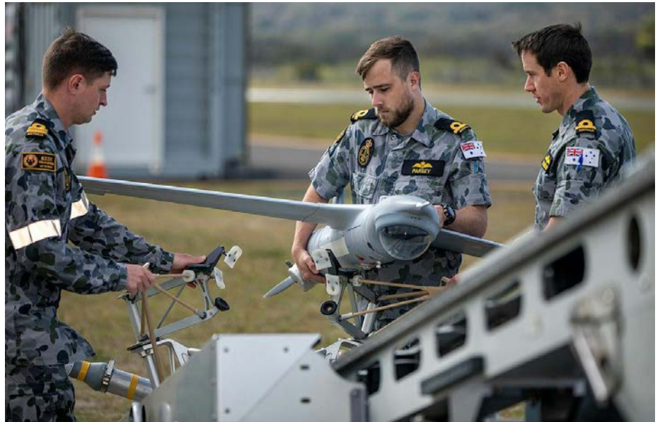
Members of the first Remote Pilot Warfare Officer course load a ScanEagle unmanned aircraft to the launcher before a flight at Jervis Bay Airfield. Defence image.
