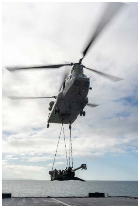
An Australian Army CH-47 Chinook helicopter lifts a M777 155mm Howitzer from Royal Australian Navy ship HMAS Choules, during Exercise Sea Explorer. Defence image.
