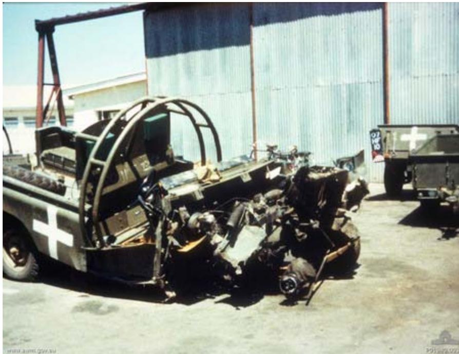
*Southern Rhodesia. British Rover equipped with mine protection gear shows extensive damage from striking a mine. There were no casualties.*
